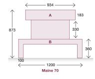
Both A and B are 300mm deep (from wall to front of unit)
