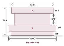
Both A and B are 300mm deep (from wall to front of unit)
