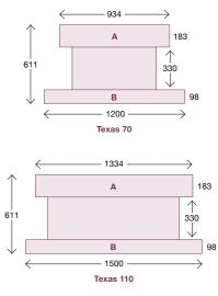
Both A and B are 300mm deep (from wall to front of unit)
